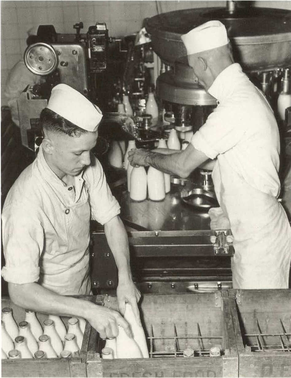
Milk was delivered at 7d a quart to the household's own container, or 8d in bottles. In this factory men remove bottles from the cap sealing machine at the rate of 4800 an hour. Pix, 5 Nov 1938.
